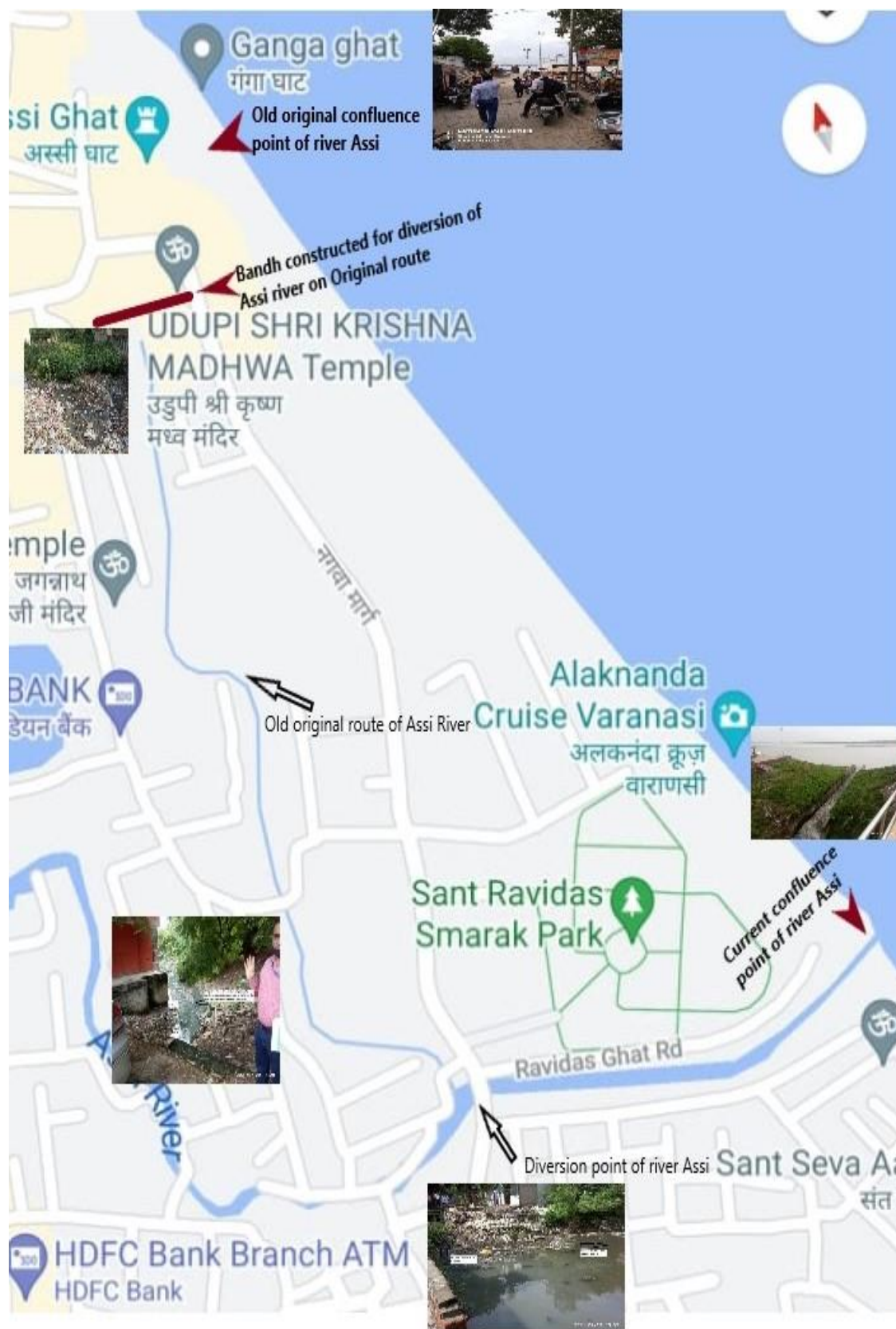
Figure 3.3. Schematic layout showing diversion of River Assi, Old channel and the present Confluence point.
