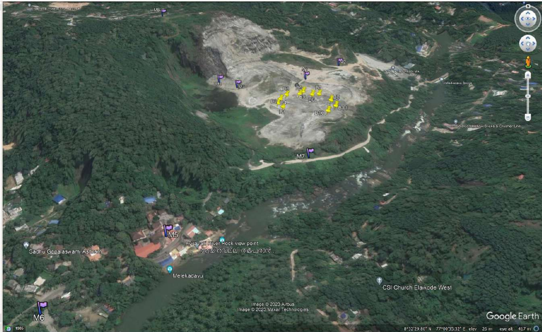
Figure 5.3.3. Google map showing location of experimental blasts and ground vibration monitoring points at granite building stone quarry of M/s POABS Granites Pvt. Ltd., Trivandrum
