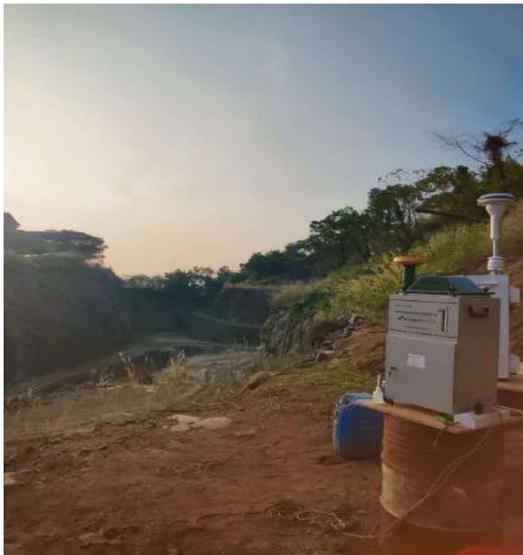
Particulate matter monitoring
