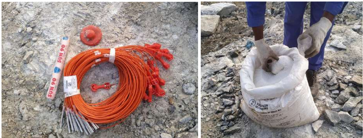
Plate 5.3.6. Emulsion explosive cartridge, Twin-det Nonel detonators and ANFO explosive
