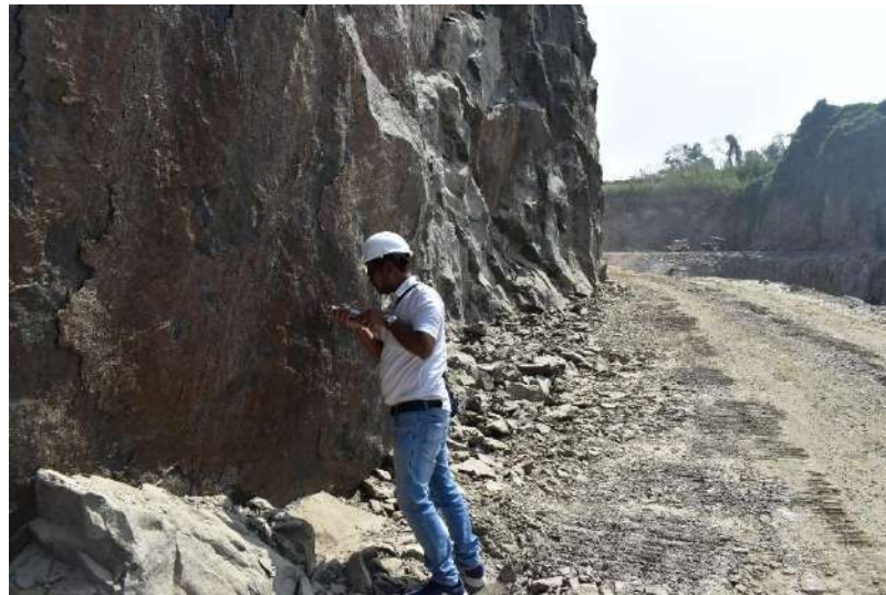
Plate 5.6.5. Assessment of rebound hardness of insitu rockmass
