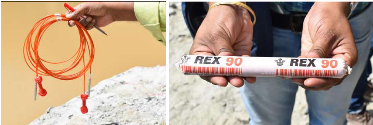
Plate 5.6.7. Nonel detonators and cartridge explosive used for charging in blastholes at the quarry
