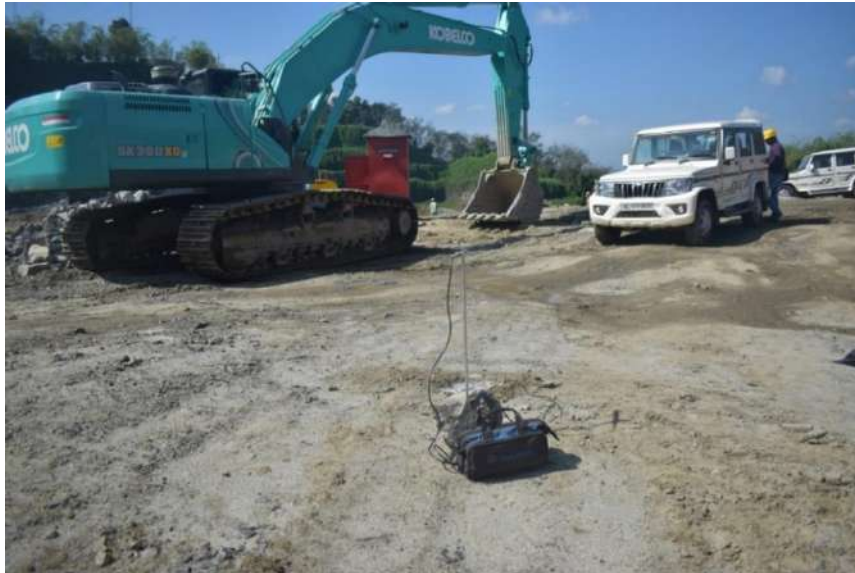
Plate 5.4.11. Monitoring of ground vibration and air overpressure within the quarry area
