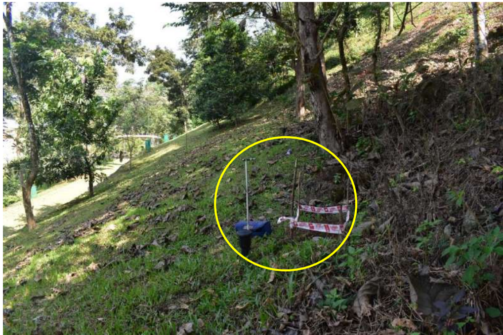
Plate 5.5.15. Monitoring of ground vibration and air overpressure in latex garden near MD's house
