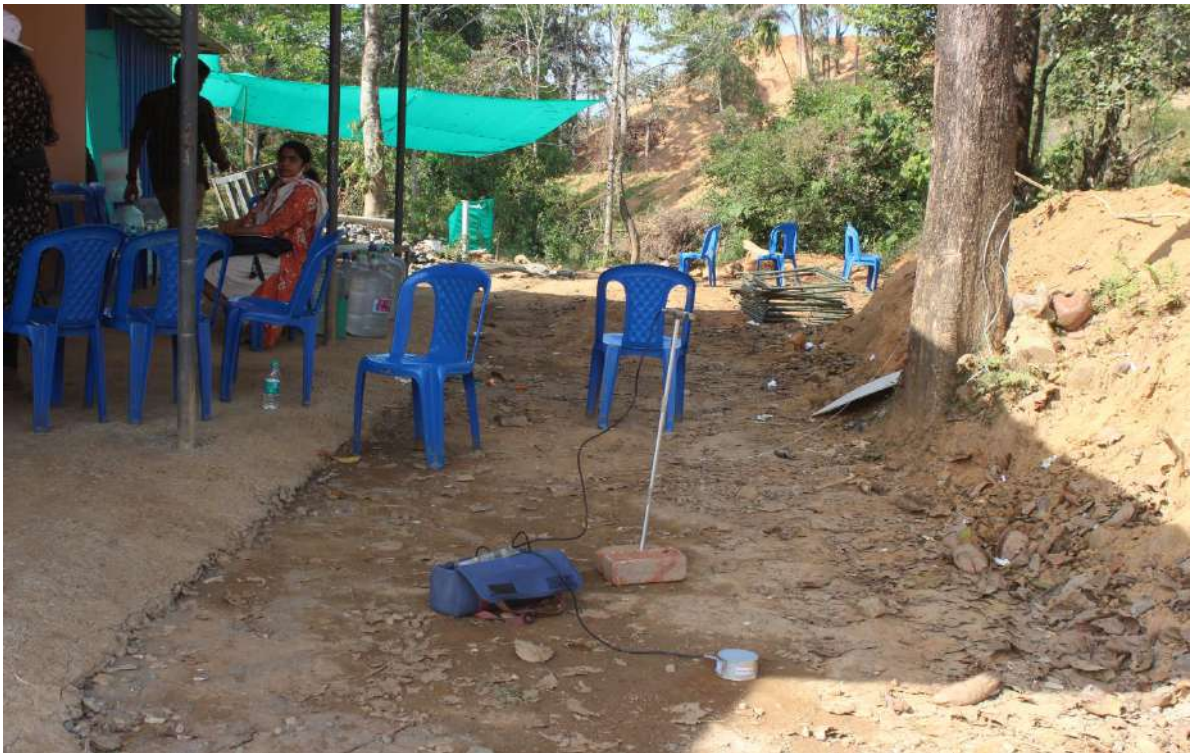
Plate 5.8.10. View of vibration monitoring at the Mine office
