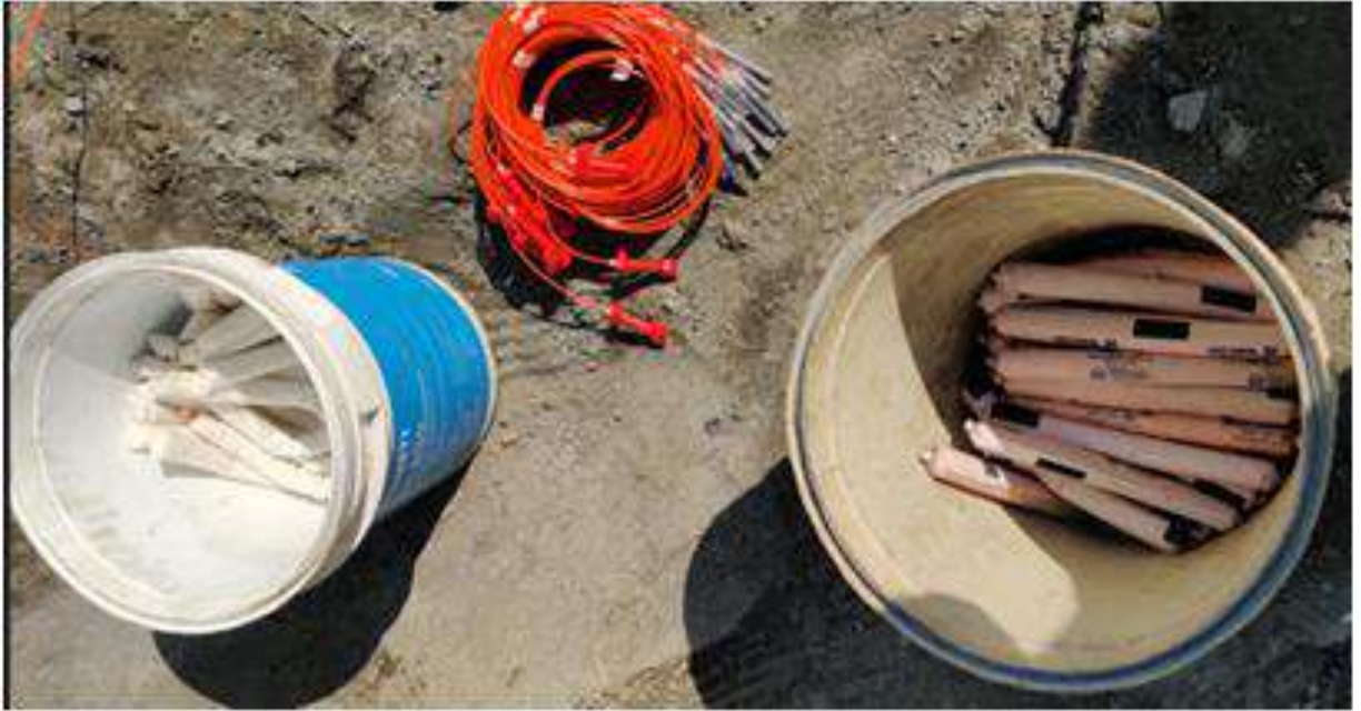
Plate 5.4.7. Emulsion explosive cartridge, ANFO cartridge and Twin-det Nonel detonators
