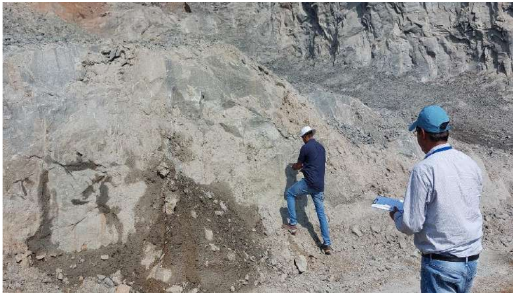
Plate 5.7.2. View of rebound hardness testing on rock surface at Granite (Building Stone) Quarry of M/S Penta Granites, Palakkad District of Kerala State
