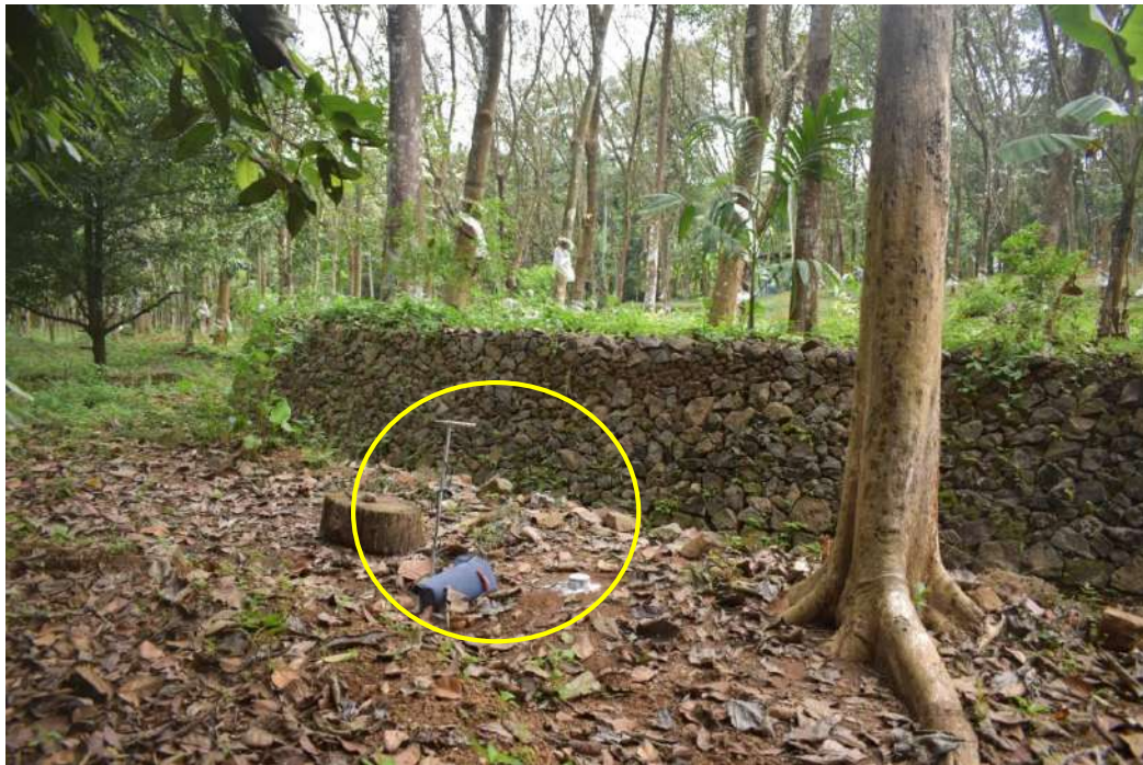
Plate 5.4.18. Monitoring of ground vibration and air overpressure in the Latex Garden of Leela's house
