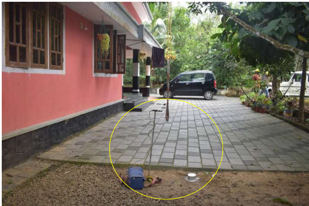
Plate 5.4.16. Monitoring of ground vibration and air overpressure at Anthru's house
