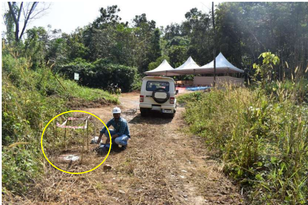
Plate 5.5.19. Monitoring of ground vibration and air overpressure near view point
