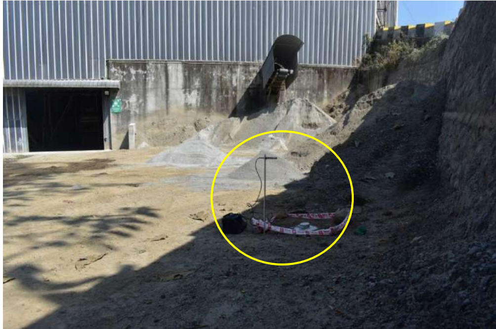
Plate 5.5.14. Monitoring of ground vibration and air overpressure near crusher plant
