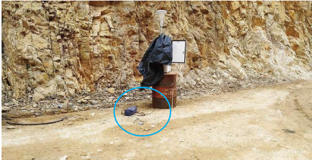
Plate 5.2.7. View of vibration monitoring point on the haul road
