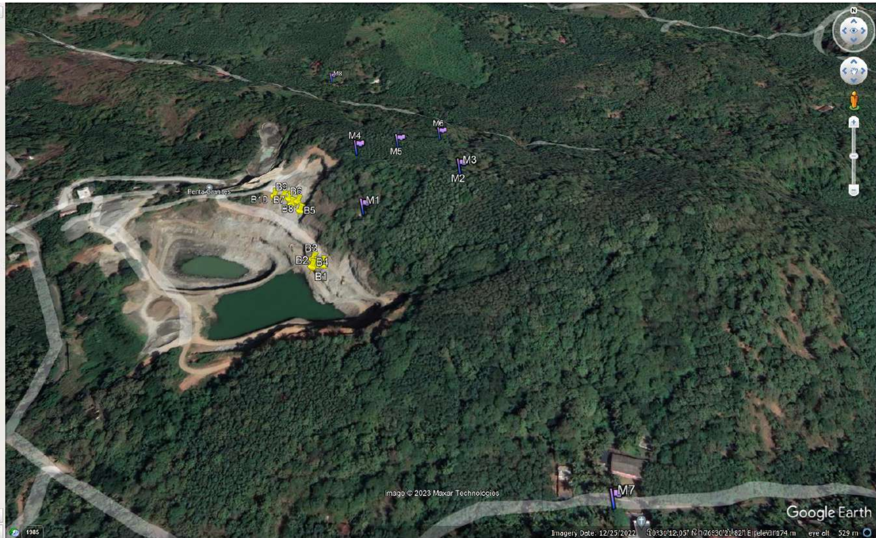
Figure 5.7.3. Google map showing locations of experimental blasts and vibration monitoring points at Granite (Building Stone) Quarry of M/s Penta Granites, Palakkad District of Kerala State
