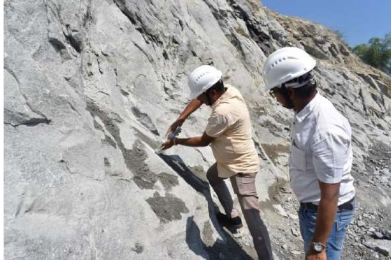
Plate 5.5.6. Assessment of rebound hardness at Rubble Stone Quarry
