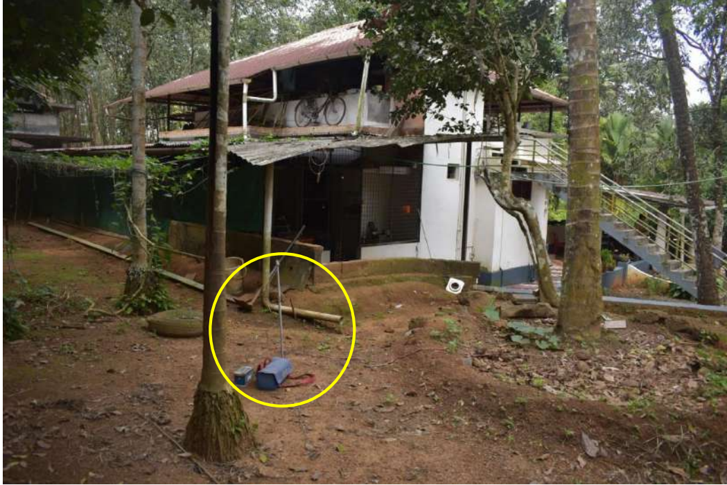
Plate 5.4.17. Monitoring of ground vibration and air overpressure at Leela's house
