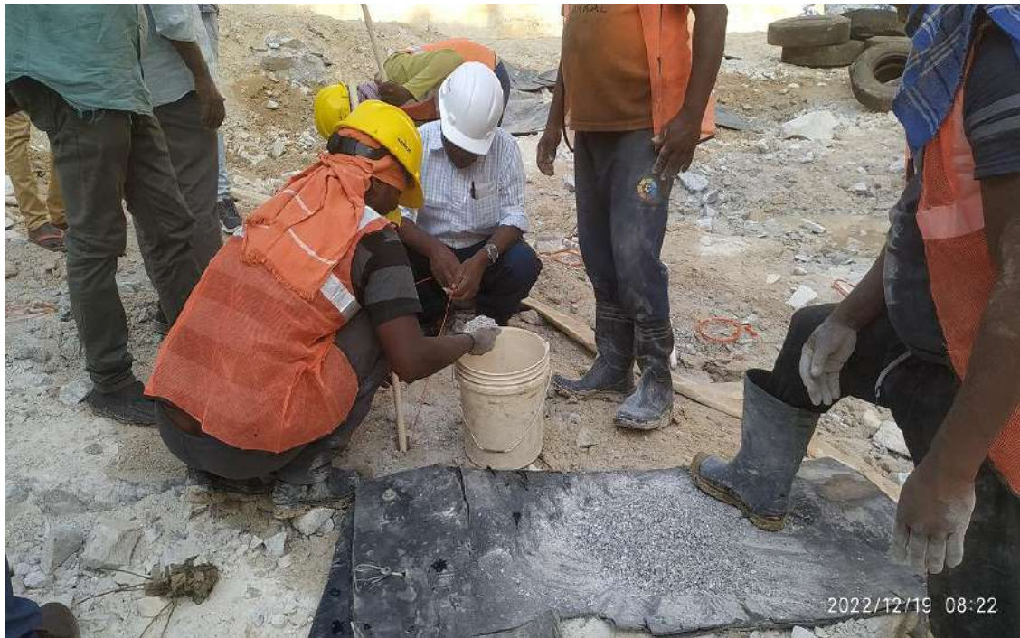
Plate 5.2.5. View of charging of holes at granite building stone quarry of Muhammad Roshen
