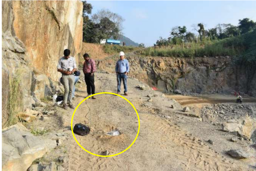
Plate 5.6.9. Monitoring of ground vibration and air overpressure at 5th Bench of the quarry
