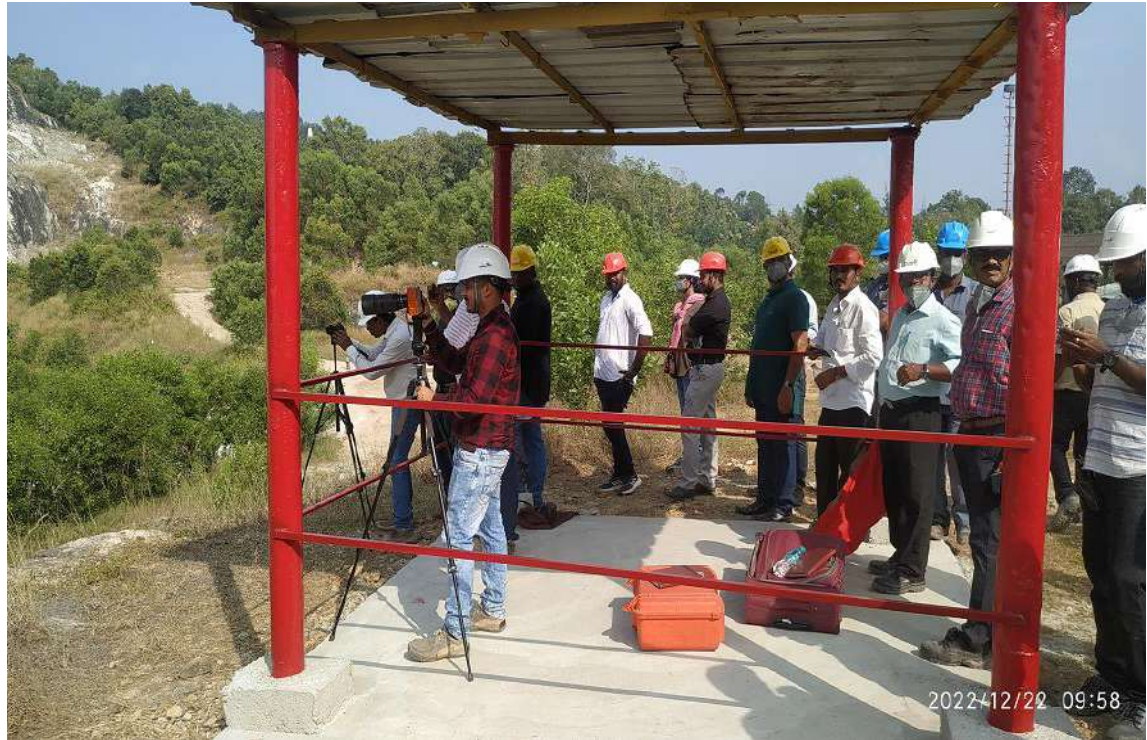
Plate 5.3.9. View of recording of blasting event using High Speed Video Camera at quarry of M/s POABS Granite Pvt. Ltd.
