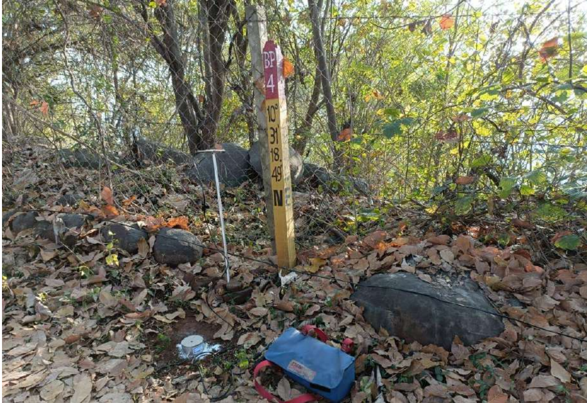
Plate 5.7.7. View of vibration monitoring at Latex Garden behind blast face
