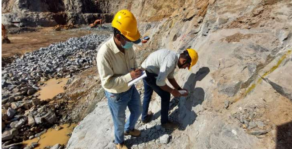
Plate 5.9.2. View of rebound hardness testing on rock surface at Granite Building Stone Quarry owned by P. M. Abdul Rahaman, Kasargod District of Kerala State
