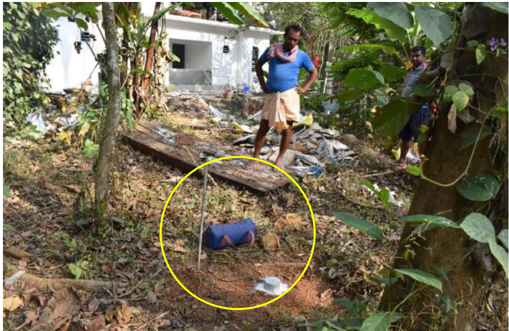
Plate 5.6.16. Monitoring of ground vibration and air overpressure Antony's house
