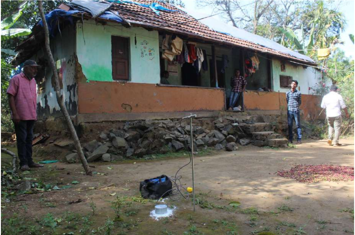
Plate 5.8.9. View of vibration monitoring at the house of Smt. Devi T. G.
