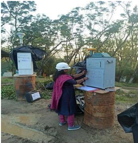
Particulate matter monitoring
