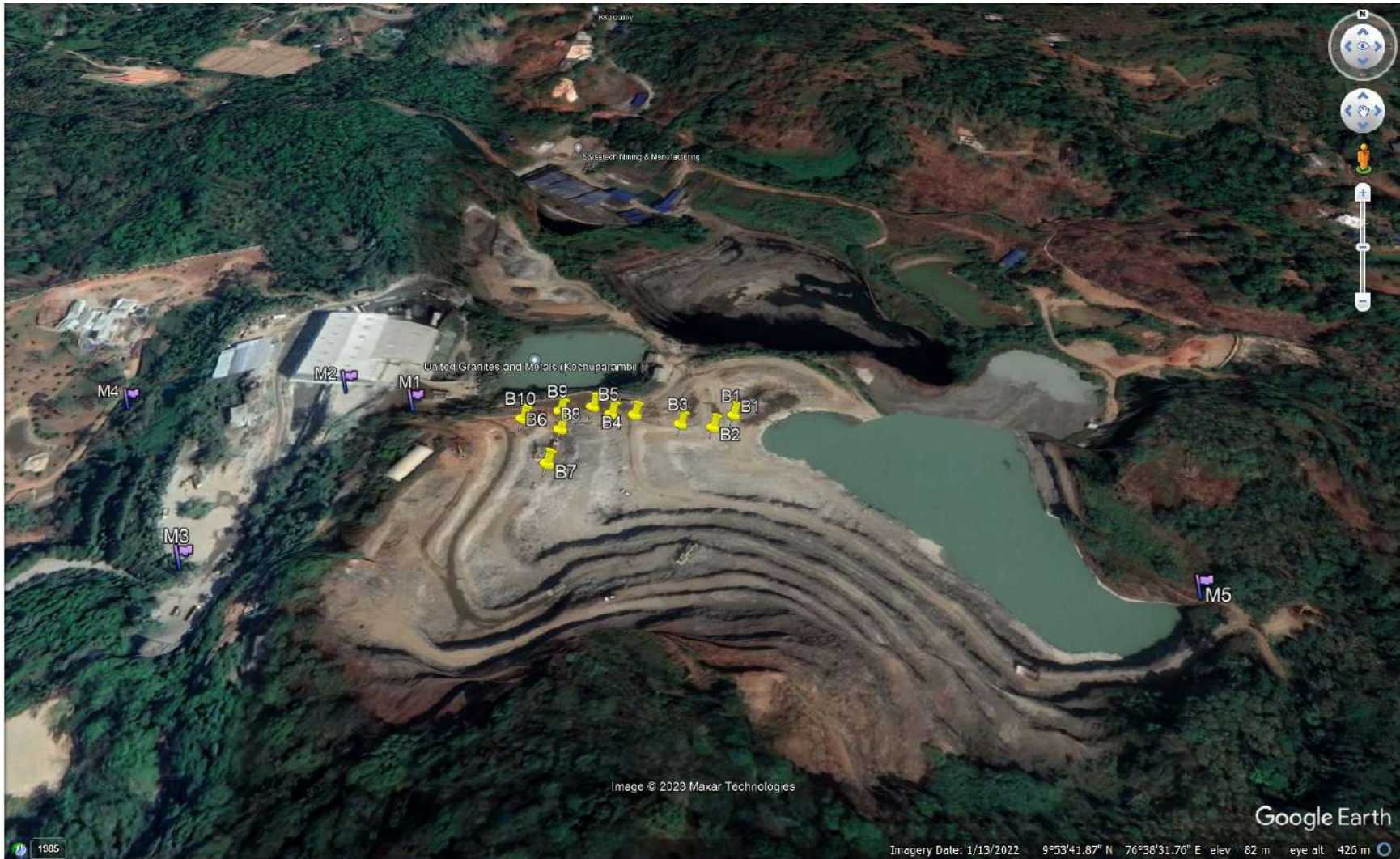
Figure 5.5.1. Google map showing location of blasts and vibration monitoring points at Rubble Stone Quarry of M/s United Granites Pvt. Ltd., Idukki District
