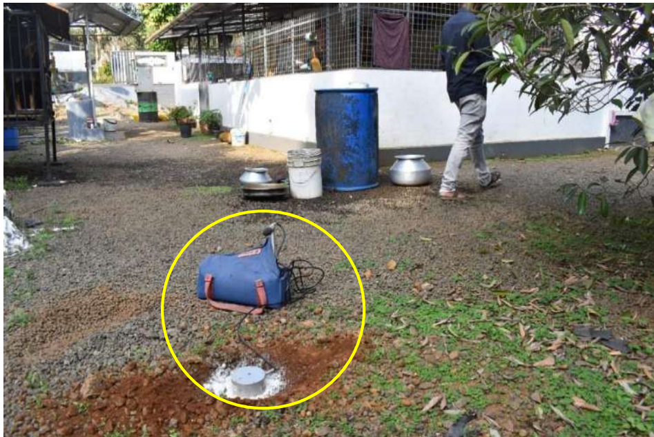
Plate 5.6.12. Monitoring of ground vibration and air overpressure near Settunath's house
