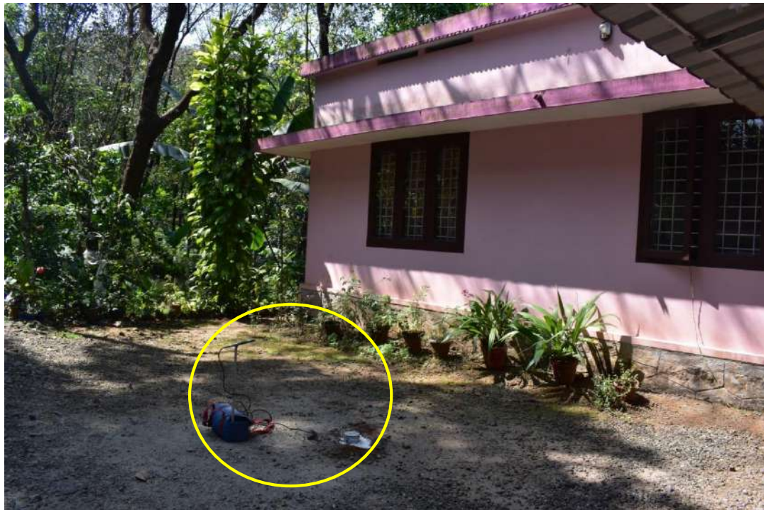
Plate 5.5.18. Monitoring of ground vibration and air overpressure at Mary's house
