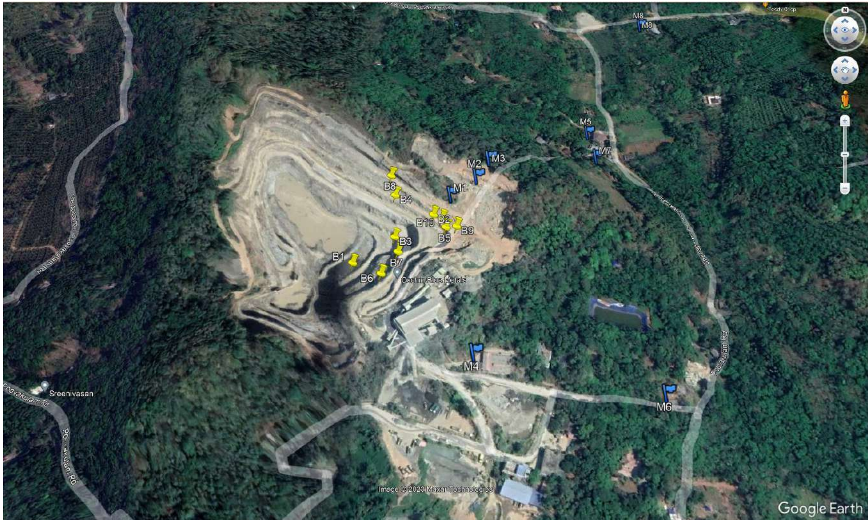
Figure 5.6.11. Google map showing location of blasts and ground vibration monitoring points at Granite Stone Quarry of M/s Blue Metal Industries Limited Kottayam District
