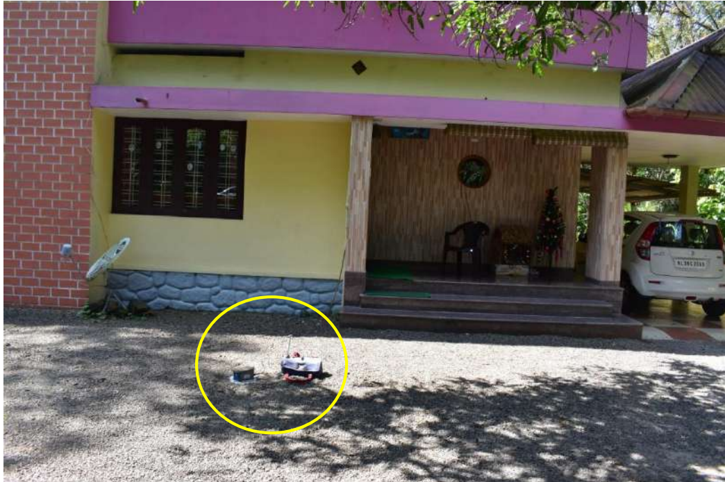
Plate 5.5.16. Monitoring of ground vibration and air overpressure at Jacob's house
