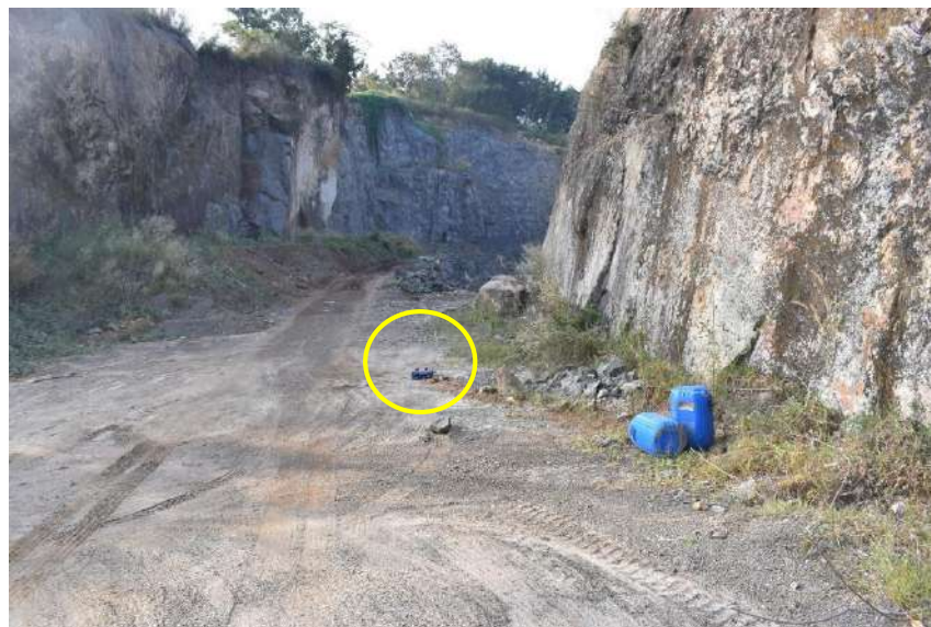
Plate 5.6.10. Monitoring of ground vibration and air overpressure inside the quarry
