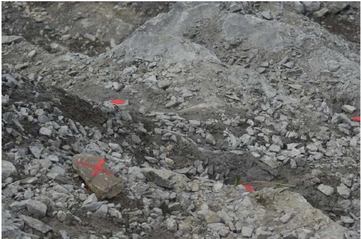
Plate 5.4.4. Marking of drill holes at Parackal Stone Quarry
