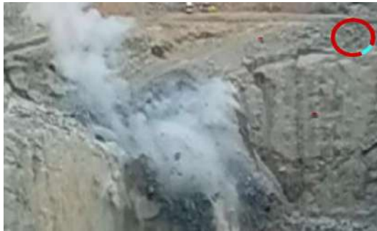
(E) Last Stage of Rock movement with flyrock
