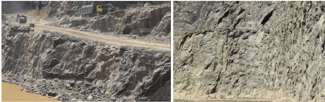
Plate 5.6.4. View of different joint sets at Granite stone quarry of M/s Cochin Blue Metal
