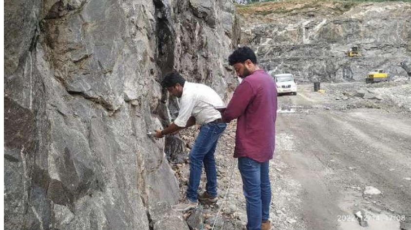
Plate 5.1.3. View of rebound hardness testing on rock surface at Granite Building Stone Quarry
