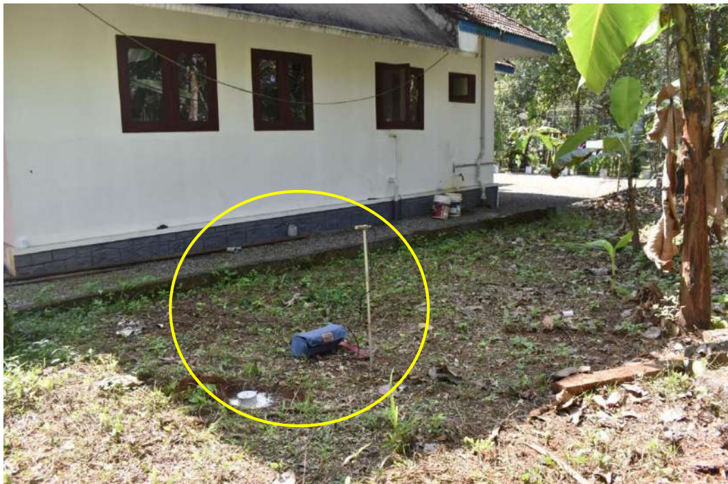
Plate 5.5.17. Monitoring of ground vibration and air overpressure at Thomas' house
