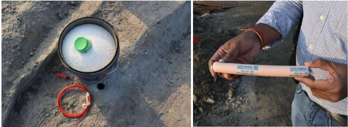
Plate 5.5.8. ANFO, Nonel detonators and cartridge explosive used for charging in blast holes at Rubble Stone Quarry
