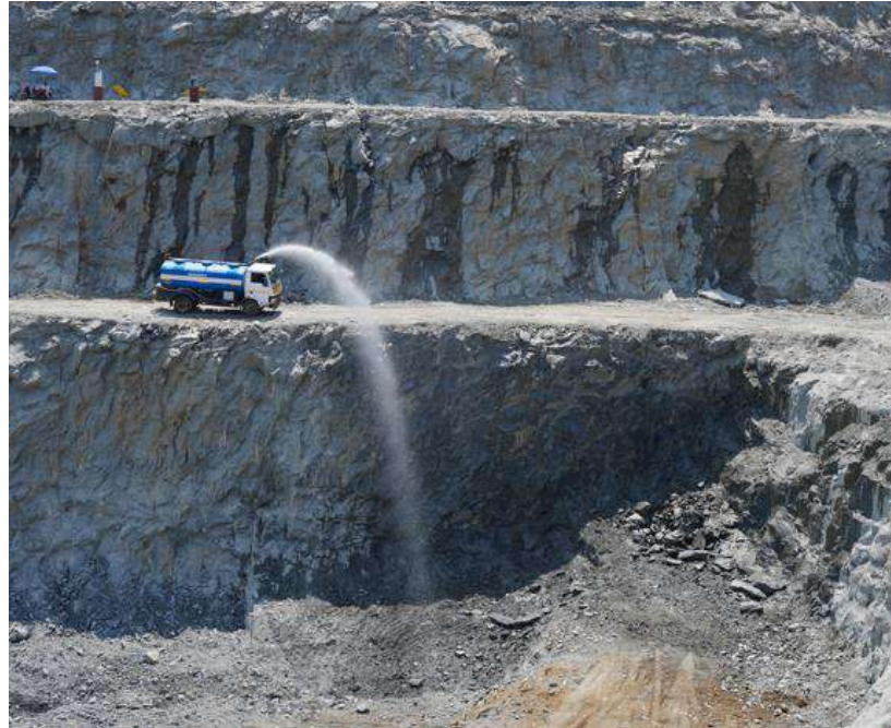
Plate 5.5.11 Water sprinkling arrangement to minimise the dust generation during blasting
