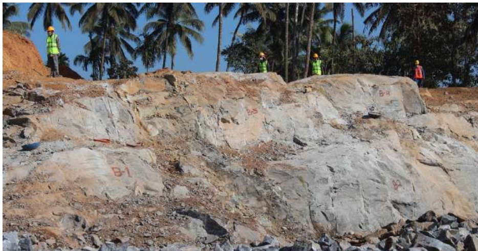
Plate 5.9.1. View showing the nature of rock deposit in Granite Building Stone Quarry owned by P. M. Abdul Rahaman, Kasaragod District of Kerala State
