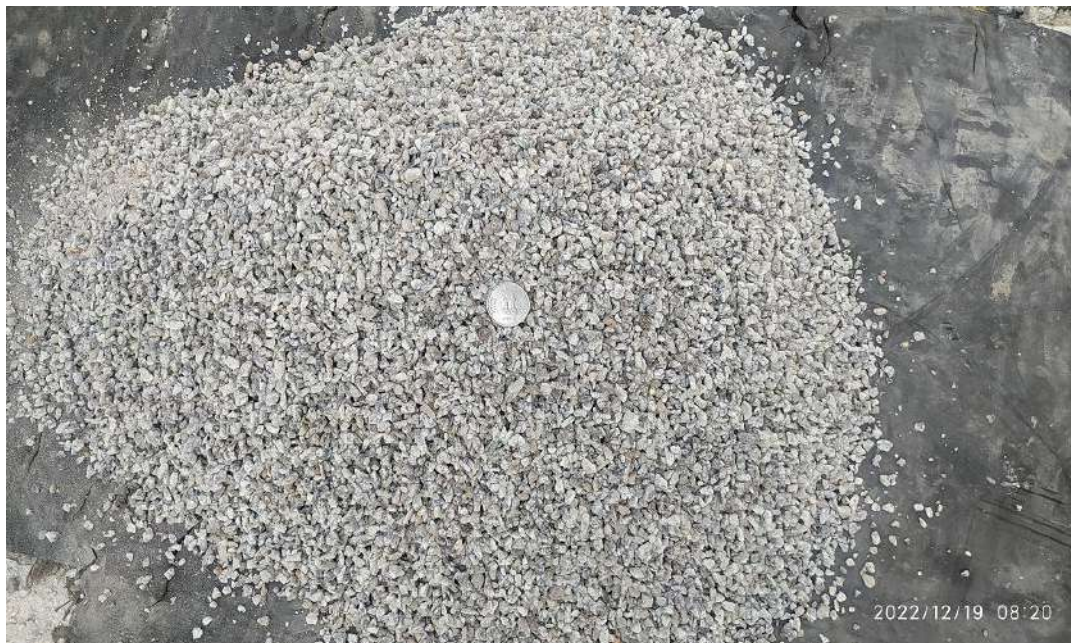
Plate 5.2.4. View of stemming material used at granite building stone quarry of Muhammad Roshen
