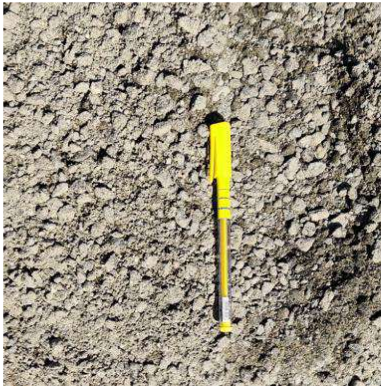
Plate 5.4.8. Stemming material for proper packing of the blast holes
